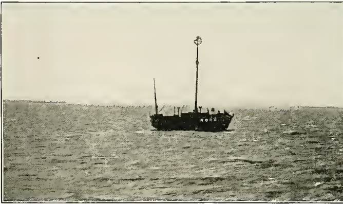
FIG. 69. — A light-ship on which men live, keeping the light on the mast burning at night, and the fog whistle blowing in foggy weather.
